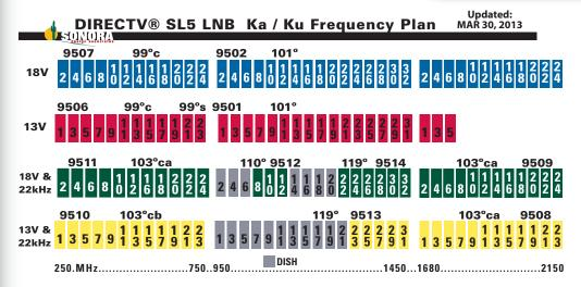
**DIRECTV®** receivers and the AIM meter are programed to measure the transponders targeted for specific zip codes. The signal meter in the receivers can be used to verify the transponders for your region.
